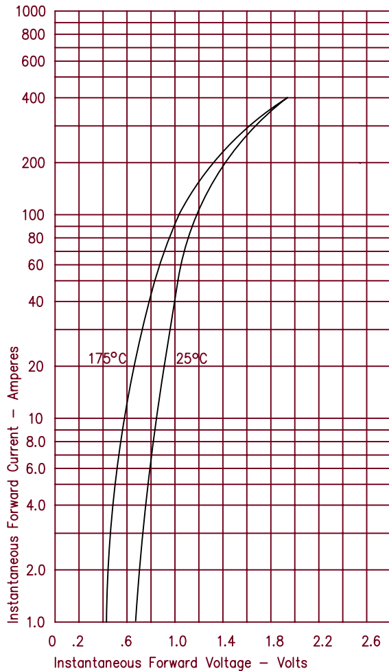
Figure 1 Typical Forward Characteristics
