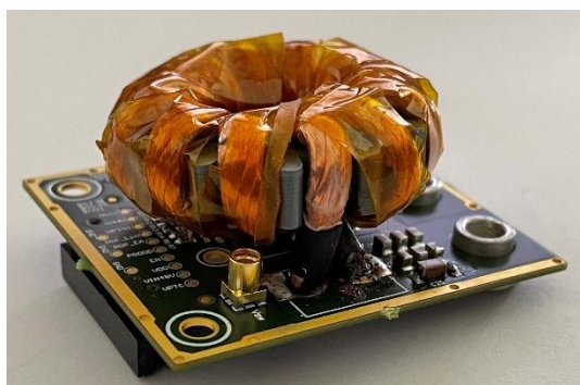
Figure 14: EPCS401 with air-core 220nH inductor.
