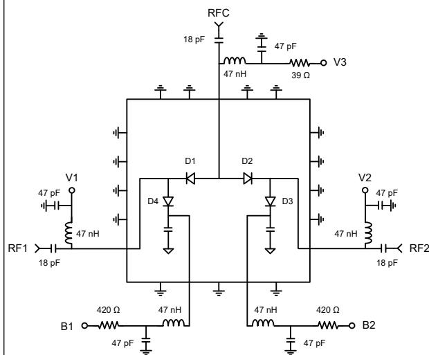
In order to safely operate at 100 W incident power, the values of the reactive components that make up the bias decoupling networks and DC blocking must be rated appropriately. Proper heat sinking is essential to safe operation under high incident power.
